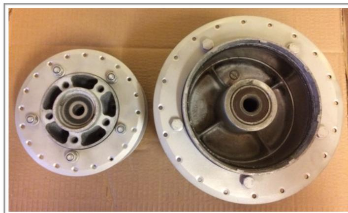
5. We will remove the wheel bearings from the hubs. We have a full set of service tools for removal of the threaded retaining rings.
